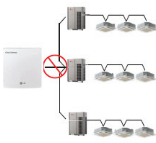
<Incorrect example : RS485 STAR format connection>
