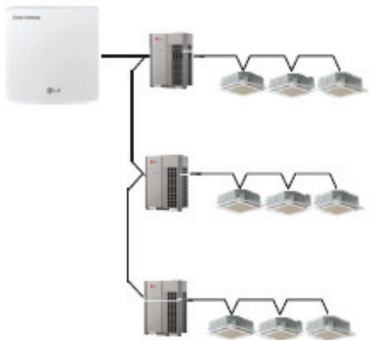
<Correct example : RS485 BUS format connection>
